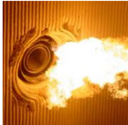
Circular – furnace wall ( Excess air 3-5%)
