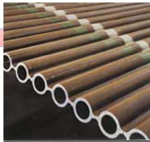
Benson boiler with a combination water wall of the former two types
